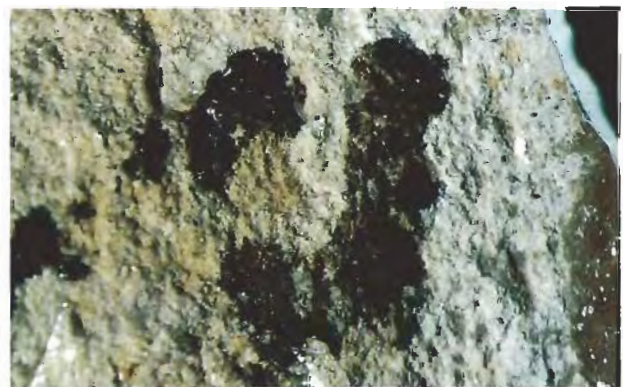
Figure 12. Black flakes of ramsdellite were sometimes visible at the interface between the opal and its matrix and may occur in the cracks in some rough and fashioned Ethiopian opal. Photomicrograph by John I. Koivula; magnified 5 \times .
