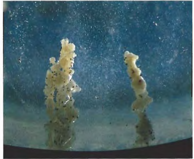
Figure 11. Rough-sided epigenetically filled "tubes," similar to those seen in some opals from Querétaro, Mexico, were observed in this 3.57 ct Ethiopian opal cabochon. Photomicrograph by John I. Koivula; magnified 15 \times .
