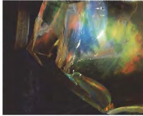
Figure 7. This piece of rough Ethiopian opal illustrates the contra luz effect: With darkfield illumination (left) no play-of-color is seen; with fiber-optic illumination from the side (right), strong play-of-color is visible. Photomicrograph by John I. Koivula; magnified 4 \times .
