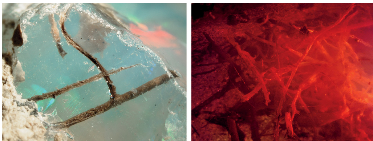
Figure 9. Irregular tube-like inclusions that appear to be fossilized plant matter occurred in both the Wollo opal (left, image width 4.4 mm) and the dyed opal (right, image width 5.0 mm) samples. Photomicrographs by S. F. McClure.
