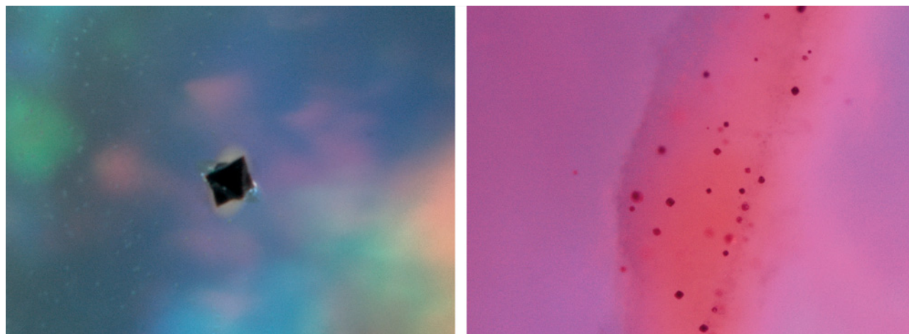
Figure 8. Both the Wollo (left) and dyed purple (right) opals showed irregular to octahedral black-appearing crystals of pyrite. Photomicrographs by N. Renfro (left, image width 0.8 mm) and S. F. McClure (right, image width 1.7 mm).
